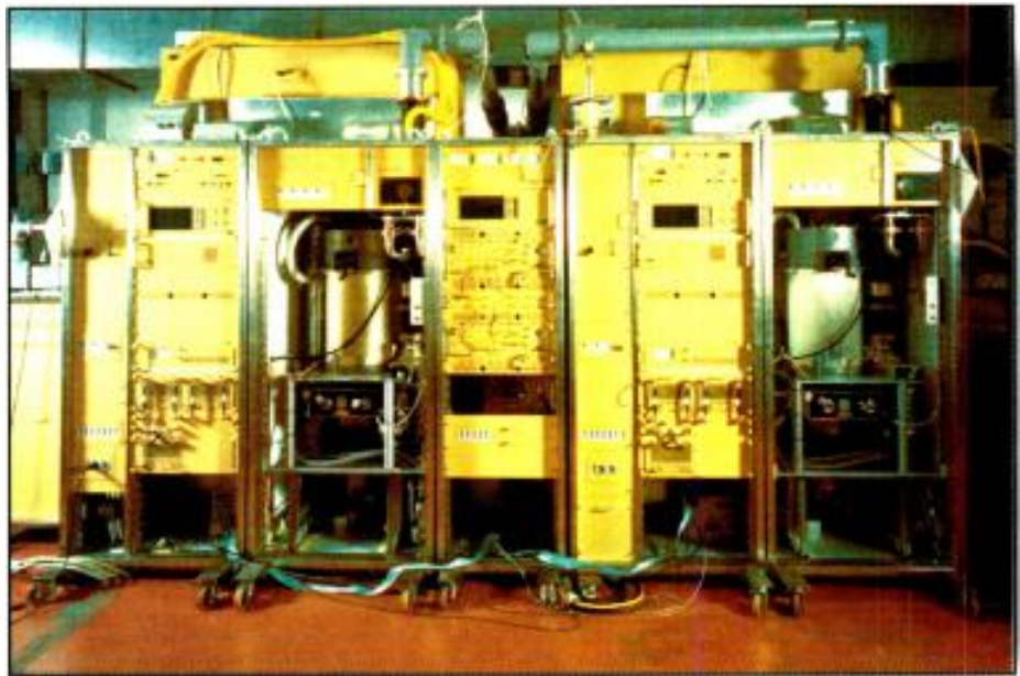
An Itelco 604K 80kW IOT undergoing final acceptance tests at the factory.
